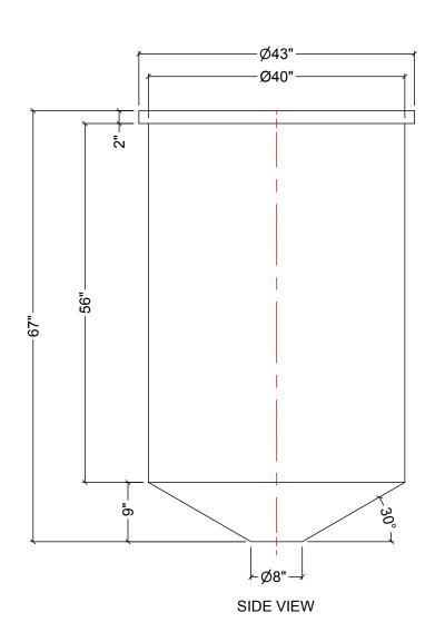
1. TANK IS MANUFACTURED TO ASTM-D-1998 STANDARD. 2. ALL DIMENSIONS ARE APPROXIMATE.
