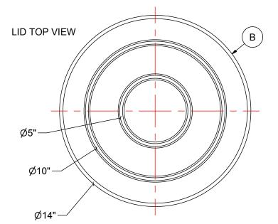
1. TANK IS MANUFACTURED FROM HDPE. (1.9 SG) 2. ALL TANK DIMENSIONS ARE SUBJECT TO A +/-3% DIMENSIONAL TOLERENCE.
